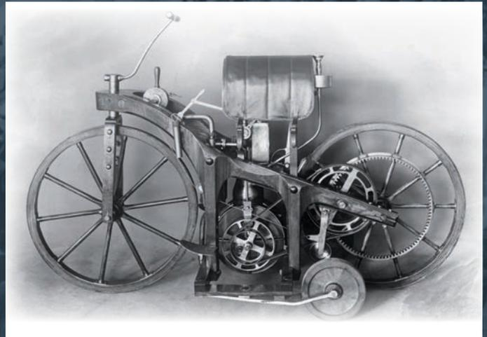
**Essential Components and Design:** The Reitwagen embodied the key elements that defined a motorcycle: a combustion engine, two wheels in-line, and a saddle for the rider. The engine, a single-cylinder, four-stroke design, was positioned beneath the rider's seat, and its power was transmitted to the rear wheel via a series of belts. The bike had no suspension, and steering was achieved by changing the wheel's direction manually.
